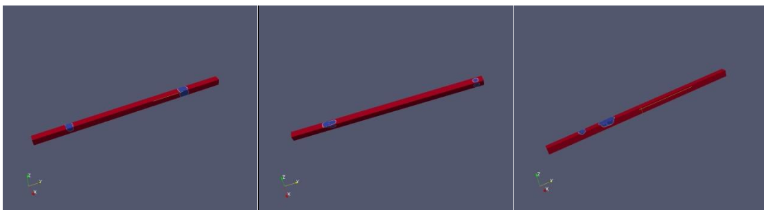
Figure 1. Liquid distribution at 0.07 seconds. (red is air and blue is liquid water)
